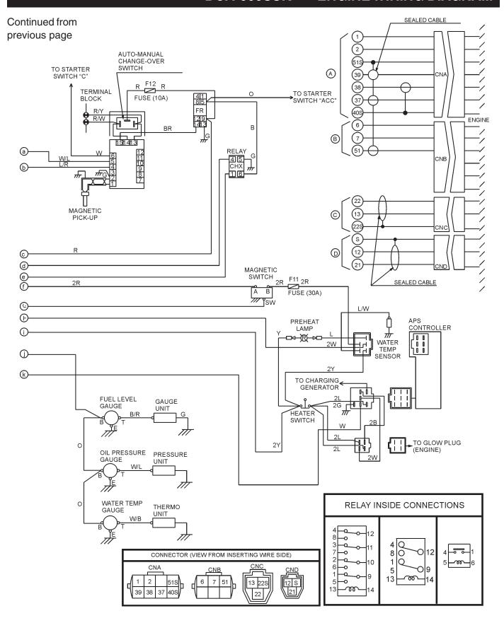
Figure 84. Engine Wiring Diagram(Continued)
